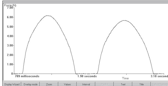
**Graph 2** The following graph shows the results when the Force Sensor was zeroed with the mass supported by the elastic.
