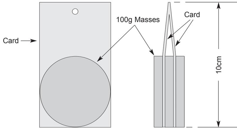
Diagram of the interrupt card with masses attached for FS1-B.
