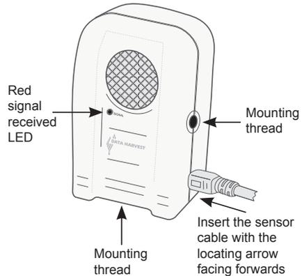
**Note:** The red signal LED on the Motion Sensor is **not** a power on indicator; it is used to indicate that a reflected signal has been received from an object.
