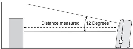
The **EASYSense** unit measures how long it takes for the ultrasonic waves to make the trip from the Motion Sensor to the object and back. Using this time and speed in air, the distance to the nearest object is determined. Any object that reflects sound can be used as a target.
