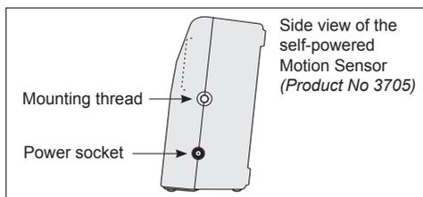
When the self-powered Motion Sensor is connected to the mains power supply the batteries will automatically be re-charged unless the Motion Sensor is taking samples. When taking samples, the current from the power supply is diverted to provide power for sampling rather than charging the batteries.
